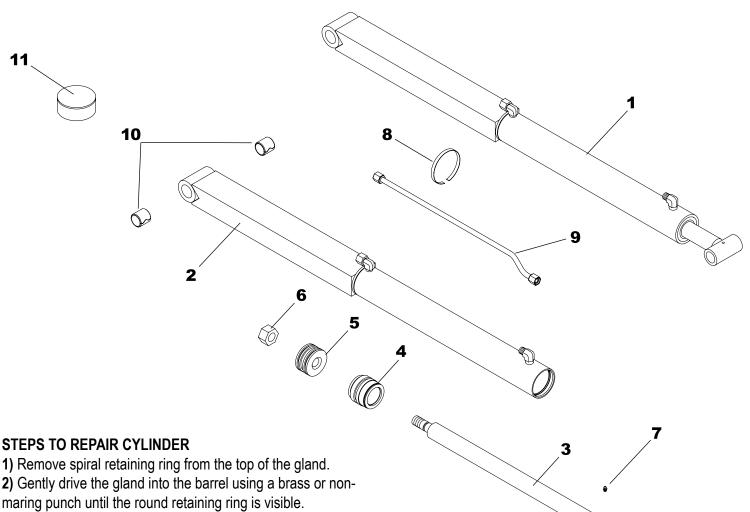
**3)** Remove the round retaining ring using a pair of long nose pliers.
