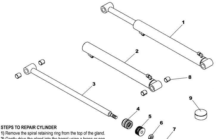
**2)** Gently drive the gland into the barrel using a brass or nonmarring punch until the round retaining ring is visible.
