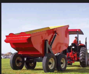
Dual action expellers are hydraulically driven to provide an aggressive and consistent spreading pattern
