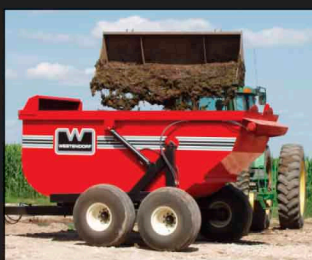
Dual action expellers are hydraulically driven to provide an aggressive and consistent spreading pattern
